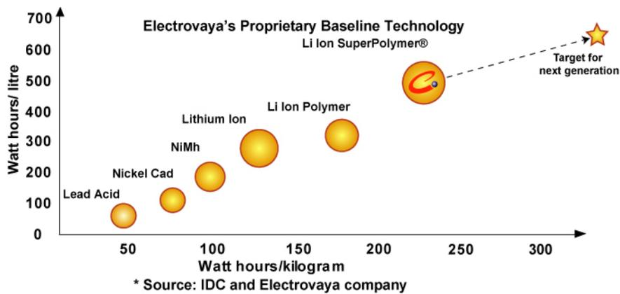
**Figure 1: Energy Comparison for Battery Technologies.**
