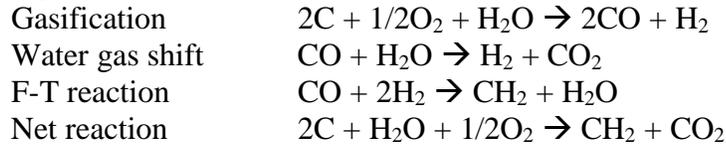
The extra hydrogen that is provided by the Water-Gas Shift can be provided by water-splitting with energy supplied from a nuclear reactor or other non-CO<sub>2</sub>-emitting source. In this case, we still provide synthesis gas as above:  $C + 1/4O_2 + 1/2H_2O \rightarrow CO + 1/2H_2$  and then provide the extra hydrogen by water-splitting:  $3/2H_2O = 3/2H_2 + 3/4O_2$ , for a net reaction of  $C + H_2O + \text{Energy} \rightarrow CH_2 + 1/2O_2$ .
