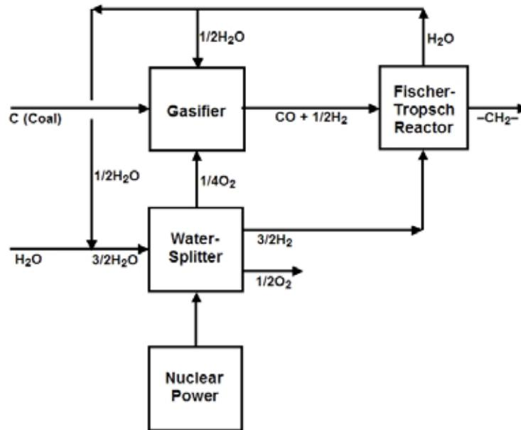
Figure 3. Coal Gasification and Fischer-Tropsch Processes Augmented with Externally Provided Hydrogen Produced by Water-Splitting.
