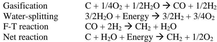
In comparison with the conventional gasification and Fischer-Tropsch sequence, only half the carbon is required, and there is no CO<sub>2</sub> produced in the conversion process. Further, oxygen is provided by the water-splitting, which avoids the need for an external oxygen supply to the gasification process, and even has some excess oxygen for potential sale. Figure 3 illustrates the complete block diagram for the idealized process.
