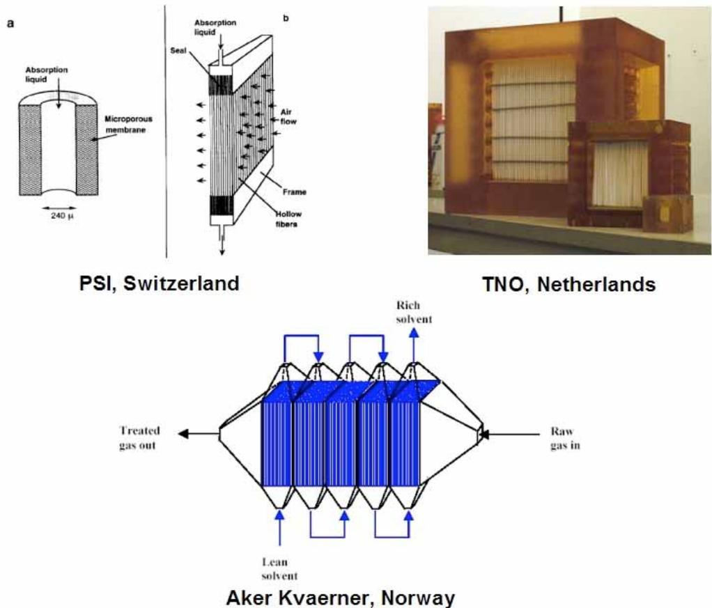
Figure 4. Sample Membrane Gas Absorption Systems and Concepts
