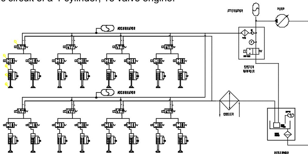
*Fig. 7: Hydraulic System Schematic for 4-Cylinder, 16 Valve Engine*
