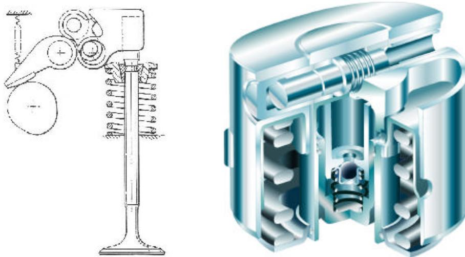
*Fig. 1: Lotus "Oscillating Cam" Early Inlet Valve Closure Mechanism (left) and Lotus-INA "Cam Profile Switching" Coaxial Tappet (right) [Courtesy INA-Schaeffler KG]*
