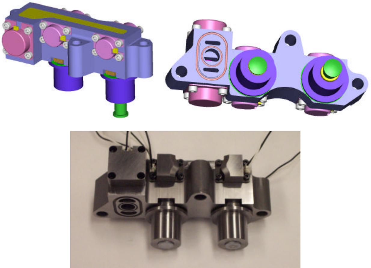
*Fig. 9: CAD Models and Photograph of AVT Sub-Module for Inlet or Exhaust Valves of a Single Cylinder*
