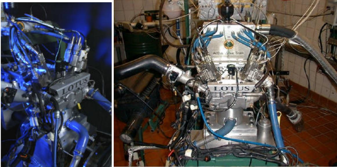
*Fig. 3: Photographs of Research AVT System fitted to a Single Cylinder Engine
