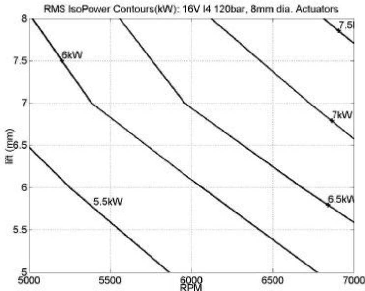
*Fig. 11(c): Predicted AVT RMS Power Consumption for 4-Cylinder 16 Valve Engine - 120bar System Pressure [High Engine Speed, High Rate of Rise for Valve High Lift]
