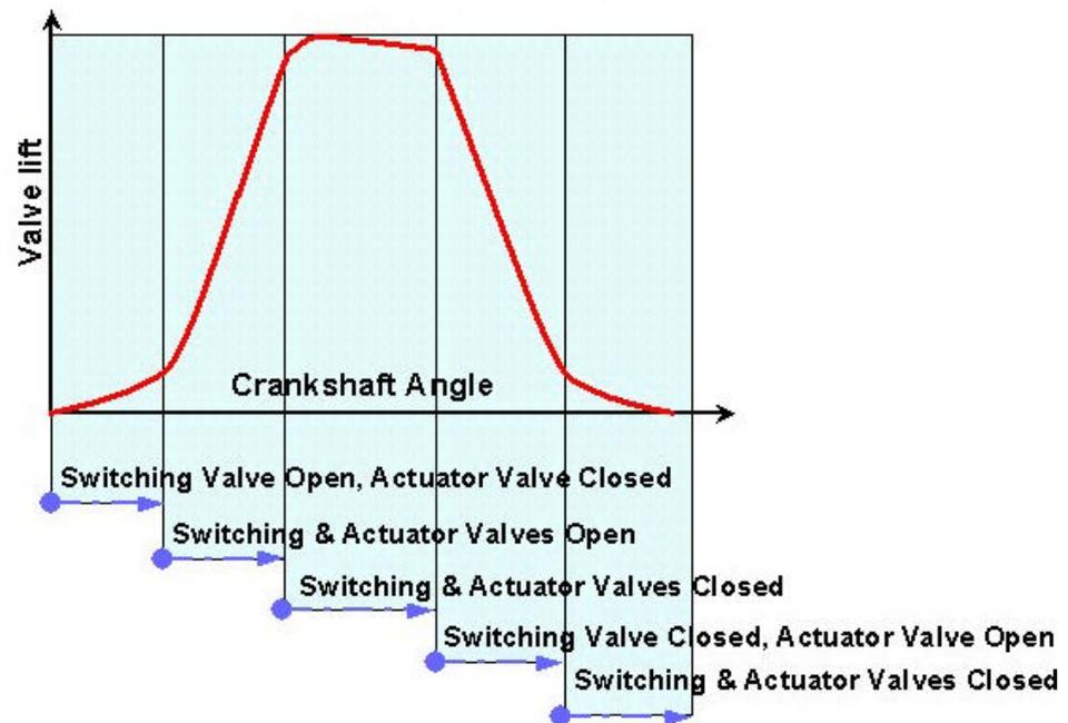
*Fig. 6: Production AVT Control Valve Sequencing versus Crank Angle*
