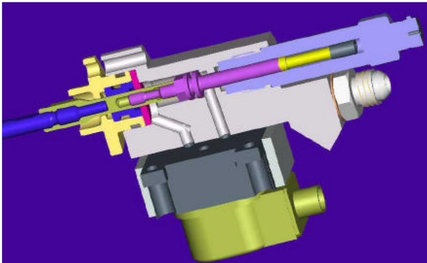
*Fig. 4: Valve Block of Research AVT Actuator (4-Way EHSV at Bottom,
