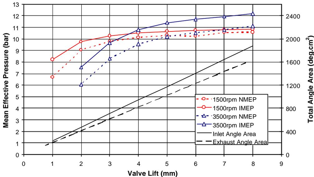
Fig. 12: Mean Effective Pressures and Angle Areas versus Lift at 1500rpm and 3500rpm using Trapezoidal Valve Profiles
