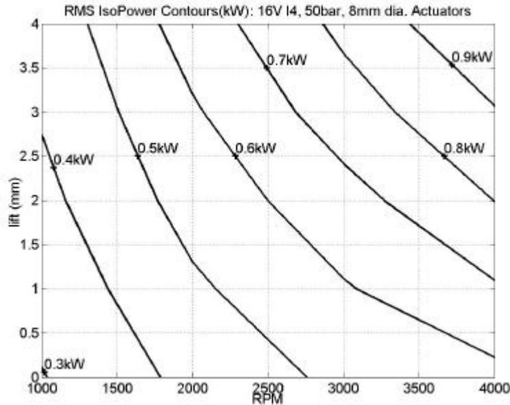
Fig. 11(a): Predicted AVT RMS Power Consumption for 4-Cylinder 16 Valve Engine - 50bar System Pressure [Low Engine Speed, Low Rate of Rise for Valve Lift]
