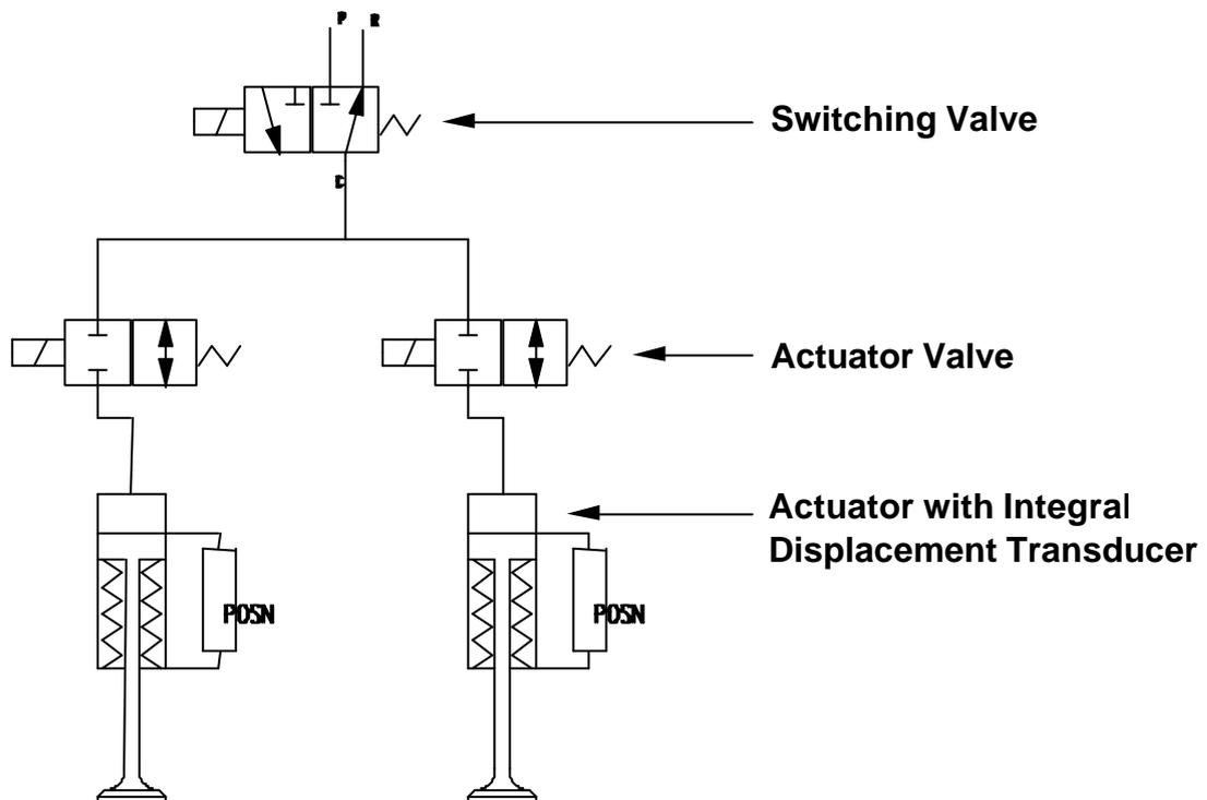
Fig. 5: Schematic of Hydraulic Circuit of Production AVT System
