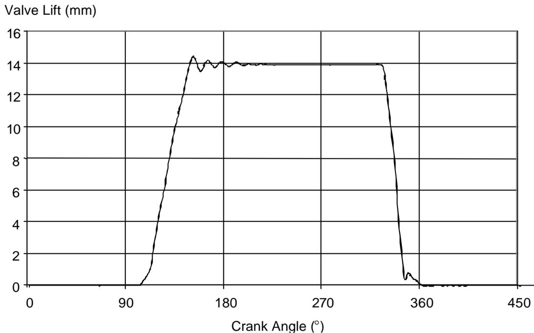
*Fig. 10: Performance of Production AVT Actuators: 1000rpm, 140bar System Pressure
