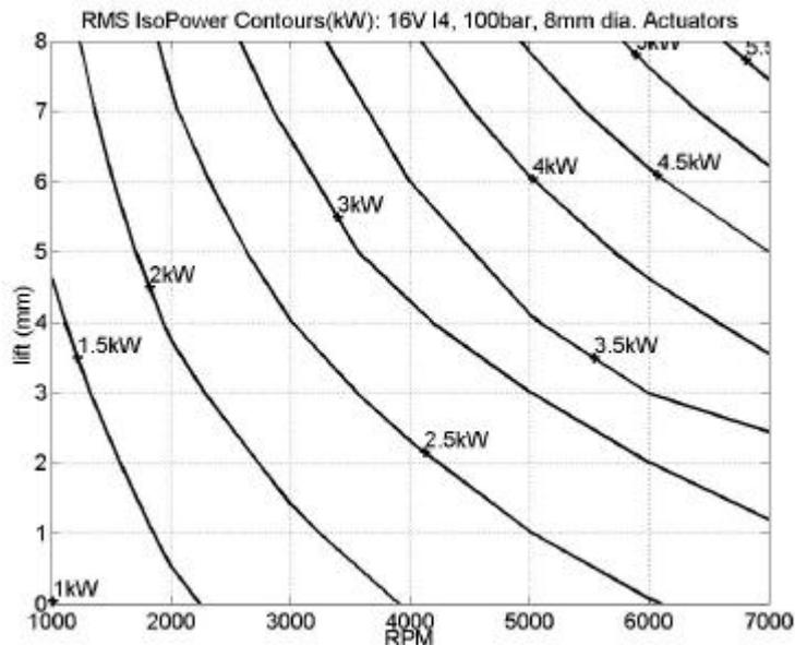
Fig. 11(b): Predicted AVT RMS Power Consumption for 4-Cylinder 16 Valve Engine - 100bar System Pressure [Full Map Operation, Intermediate Rate of Rise for Valve Lift]
